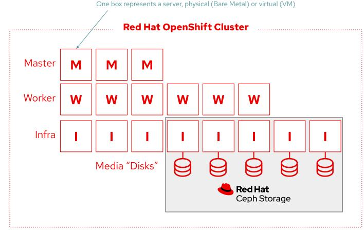
Example of an OpenShift Cluster with 3 Master-, 6 Worker and 8 Infra-Nodes. Ceph is installed (by Rook) on the Infra-Nodes as a 5-Node Cluster, leveraging Media (Disks) locally attached to the Infra-Nodes.
